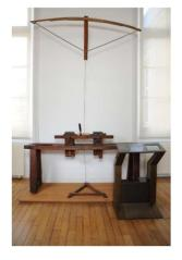
John Horsley, in his book on Maritime Tools, has a sketch of a traditional workshop lathe with a heavy bed of wooden beams powered by a pole suspended horizontally across the ceiling of a workshop.
