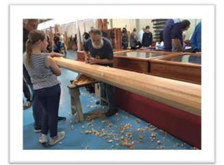
Once the timber was glued up we effectively had two square structural beams. These were then tapered from the bottom to the top, the heels being left square for the first 1.0 metre, and the top 1.8 metres was also left square. The 9-11 metres in between was marked out for 8 equally spaced sides. It must be remembered that these masts are tapered, and it is not a straight taper either, it's rather like a Greek column, so the 8 sides
