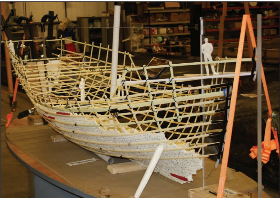
Scale model of the Newport Ship made from digital recordings.
